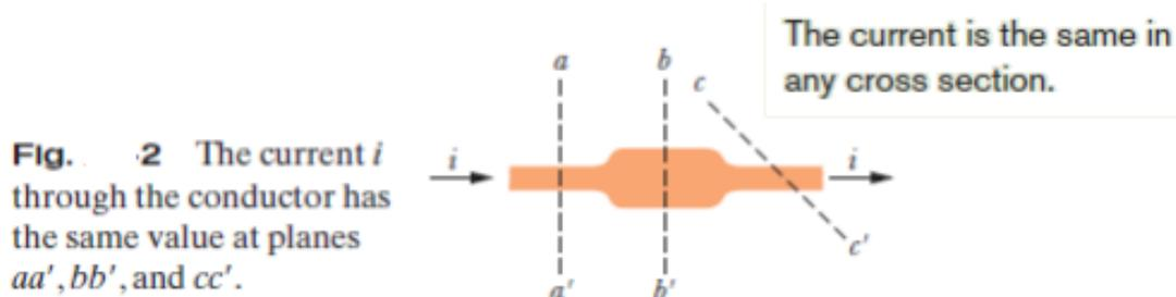
**Fig. 2** The current  $i$  through the conductor has the same value at planes  $aa'$ ,  $bb'$ , and  $cc'$ .
