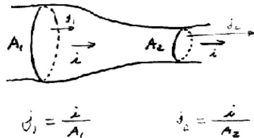
Figure below shows how current density can be represented with a similar set of lines, which we can call streamlines.
