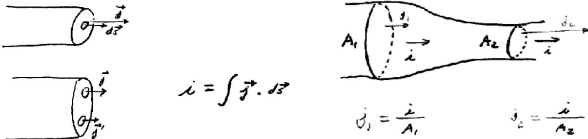
Figure below shows how current density can be represented with a similar set of lines, which we can call streamlines.
